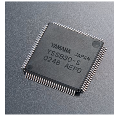
Yamaha's Exclusive YSS-930 32-Bit Floating Point Quantization LSI
